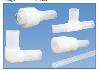
Purflon® is manufactured using ultra high purity PFA resin. A complete system of SDR pipe, valves and fittings are available in 20 - 32mm. Purflon® can be joined in the field using Asahi/America's SP series of IR welding equipment. Purflon® is designed for critical applications including ultrapure water and ultrapure chemical transfer at elevated temperatures.
