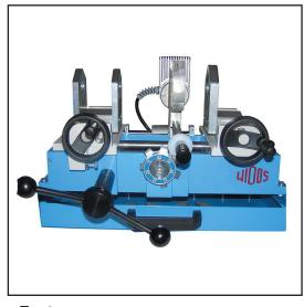
20mm - 75mm (1/2" - 2-1/2") Size Range Single wall **Piping** PE, PP, PVDF **Materials** 110V Power
