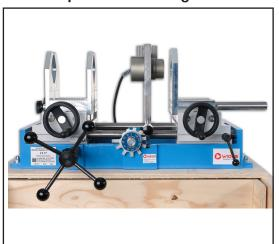
20mm - 125mm (1/2" - 5") Size Range Single wall **Piping** PE, PP, PVDF **Materials** 110V Power
