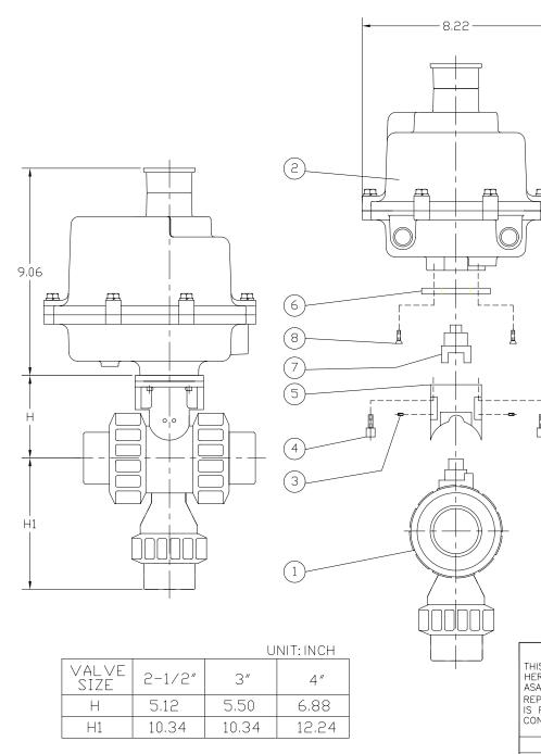
NOTE. The shape and appearance of assembly differ a little with nominal size compared to this drawing.
